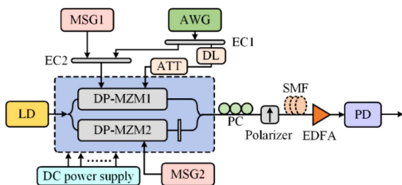
Fig. 2. Experimental setup of the proposed system. MSG, microwave signal source; AWG, arbitrary waveform generator; ATT, electrical attenuator; DL, electrical delay line; SMF, single-mode fiber.
