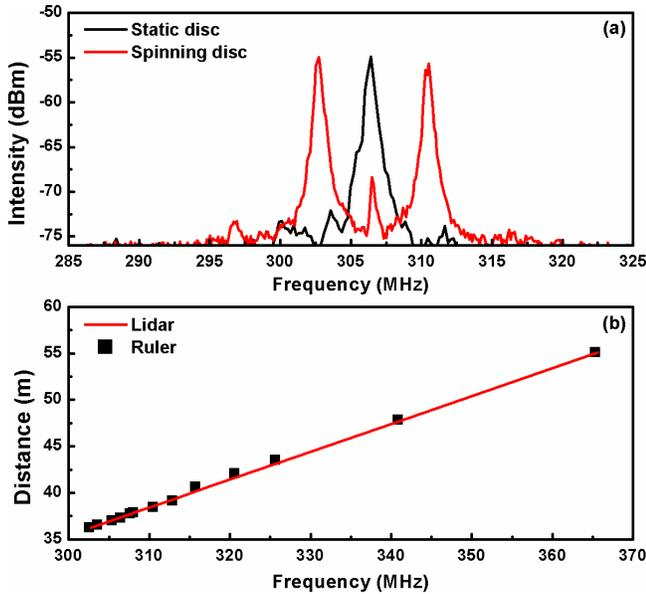
Fig. 3. (a) The de-chirped signal of the proposed DSB lidar spectra. (b) The distance measured by the Lidar (red line) and the Ruler (squared scatters).
