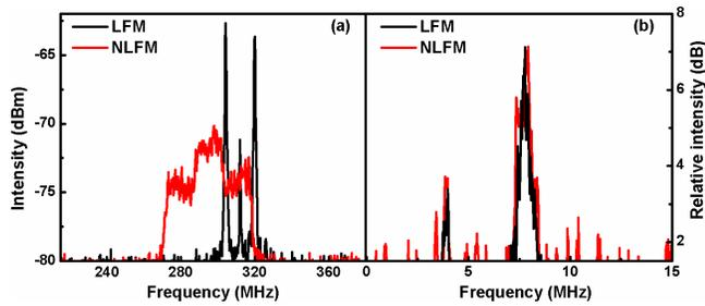
Fig. 5. (a) The dual-tone signal for LFM (black line) and NLFM (red line) (b) The difference frequency signals in the DSB lidar.
