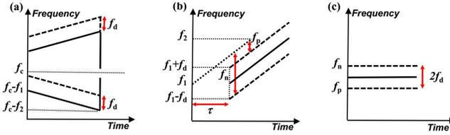
Fig. 2. Illustration of the signal evolution in the DSB lidar with a saw-tooth FMCW signal. (a) The instantaneous frequencies of the optical DSB signal (solid lines) and the reflected light experienced a Doppler shift (dashed lines). (b) The electrical signal generated by the PD (solid or dashed lines) and the saw-tooth FMCW signal from the AWG used for de-chirping (dotted line). (c) The de-chirped signal for static targets (solid line) and moving targets (dashed lines).
