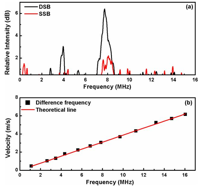
Fig. 4. Velocimetry via frequency mixing in the DSB lidar. (a) The frequency-mixing spectra in the DSB lidar and the SSB lidar. (b) The measured and theoretical frequencies for different velocities in the DSB lidar.
