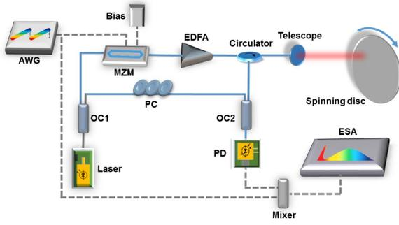
Fig. 1. Experiment setup of the proposed DSB lidar. The solid blue lines are optical fibers and the dashed gray lines are electrical cables. OC: optical coupler; PC: polarization controller; MZM: Mach-Zehnder modulator; EDFA: erbium doped fiber amplifier; AWG: arbitrary waveforms generator; ESA: electrical spectra analyzer; PD: photodetector.
