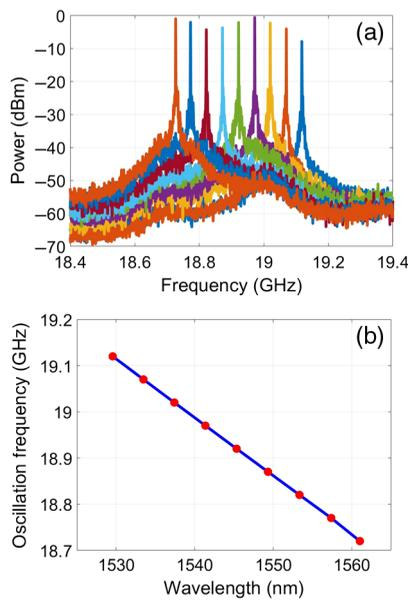
**Fig. 4** Frequency tunability of the proposed OEO. (a) Electrical spectra with a span of 1 GHz and an RBW of 30 kHz when the TLS wavelength decreases from 1561.02 to 1529.56 nm. (b) Relationship between the OF and the TLS wavelength.
