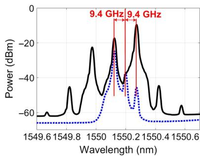
**Fig. 2** The optical spectra of the proposed OEO. Blue dotted line: the opened OEO when the RF port of the PM is disconnected. Black solid line: the closed OEO loop.
