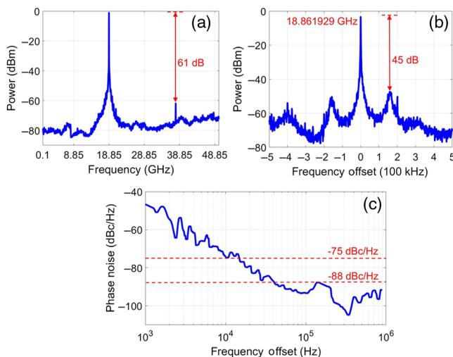
**Fig. 3** Electrical spectra and phase noise of the proposed OEO. (a) Electrical spectrum with a span of 50 GHz and an RBW of 30 kHz. (b) Electrical spectrum with a span of 1 MHz and an RBW of 100 Hz. (c) Single sideband phase noise with a frequency offset ranged from 1 kHz to 1 MHz.
