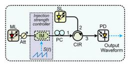
Fig. 2. Experimental setup of the proposed reconfigurable radar waveform generator based on an optically injected semiconductor laser. ML: master laser, Att: optical attenuator, IM: intensity modulator, S(t): control signal, PC: polarization controller, CIR: optical circulator, PD: photodetector.
