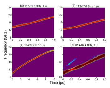
Fig. 6. STFT analysis of the generated LCMWs with (a) varied bandwidth, (b) central frequency, (c) temporal duration, and (d) frequency band.
