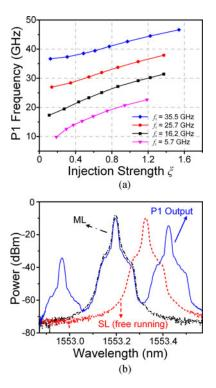
Fig. 3. (a) P1 frequency  $f_o$  as a function of the injection strength  $\xi$  for different detuning frequencies  $f_i$ . (b) Optical spectra of the injection light (black), the free-running slave laser (red), and the injected slave laser (blue) when  $(f_i, \xi)$  equals to (16.2 GHz, 1.09).
