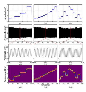
Fig. 4.  $(\alpha$ -i) Measured control signal S(t),  $(\alpha$ -ii) measured temporal waveform,  $(\alpha$ -iii) the recovered instantaneous frequency.  $\alpha$  equals to a, b and c, for generating stepped linear sequence with a length of 4, 10 and Costas sequence with a length of 10.
