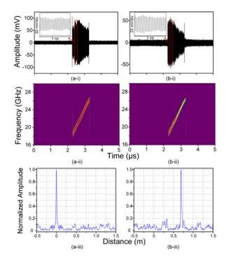
Fig. 10. (a-i) Temporal waveform, (a-ii) STFT analysis and (a-iii) autocorrelation of the transmitted signal. (b-i) Temporal waveform, (b-ii) STFT analysis of the received signal and (b-iii) correlation between transmitted/received waveform. (Insets: zoom-in views in temporal duration of 1ns).
