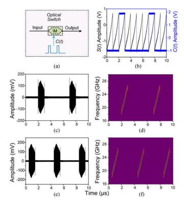
Fig. 8. (a) Schematic of the optical switch, (b) measured control signal S(t) (black) and switching signal C(t) (blue), (c) measured waveform and (d) STFT analysis of the generated linearly chirped pulse trains with a repetition rate of 200 kHz, (e) measured waveform and (f) STFT analysis of the generated pulse trains with a repetition rate of 250 kHz.
