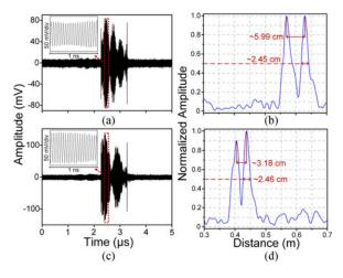
Fig. 11. Temporal waveforms the received signals when the distance between the two targets is (a) 5.99 cm and (b) 3.18 cm, the cross-correlation results when the distance between the two targets is (c) 5.99 cm and (d) 3.18 cm. (Insets: zoom-in views in temporal duration of 1ns).
