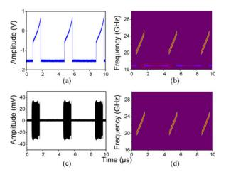
Fig. 7. (a) Measured control signal S(t), (b) STFT analysis of the generated linearly chirped pulse trains before HPF, (c) measured waveform and (d) STFT analysis of the generated linearly chirped pulse trains after HPF.
