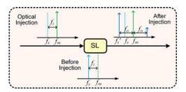
Fig. 1. Schematic diagram of an optically injected semiconductor laser and its spectral characteristic in period-one state. SL: slave laser.
