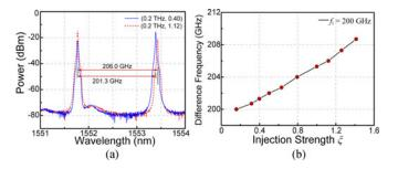
Fig. 12. Measured results when  $f_i = 200 \text{ GHz}$ . (a) Output spectra when  $\xi$  equals to 0.40 (blue) and 1.12 (red), (b) Measured difference frequency  $f_o$  as a function of the injection strength  $\xi$ .
