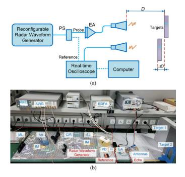
Fig. 9. (a) Schematic setup and (b) photograph of a radar system based on an optically injected semiconductor laser. PS: power splitter, EA: electrical amplifiers, AWG: arbitrary waveform generator.
