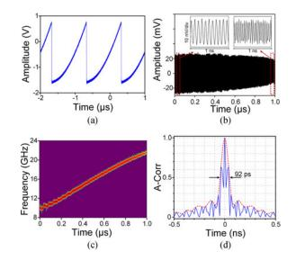
Fig. 5. (a) Measured control signal S(t) with three periods, (b) measured waveform of the generated LCMW with one period (Insets: zoom-in views in temporal duration of 1 ns), (c) recovered instantaneous frequency, (d) calculated autocorrelation result.
