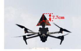
Fig. 5. The imaging target of UAV with a metallic corner reflector.
