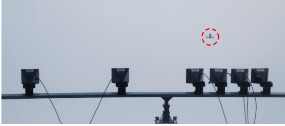
Fig. 6. The experimental detection scenario with a single target located to the right of the boresight.
