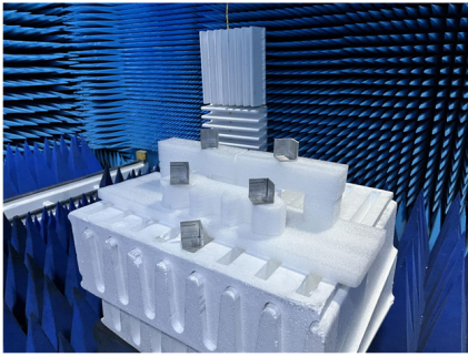
Fig. 9. Photograph of the 3-D imaging scenario of a U-shaped complex target.
