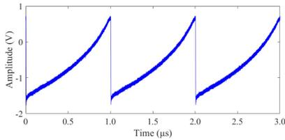
Fig. 3. The electric control signal  $S(t)$  with a near-saw tooth profile for the injection-strength controller.
