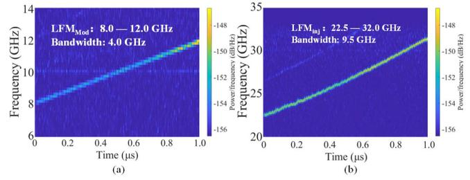
Fig. 4. The instantaneous frequency-time diagram of the LFM signal by beating the optical spectrum of (a): the blue line in Fig. 2(a), and (b): the red dotted line in Fig. 2(c).
