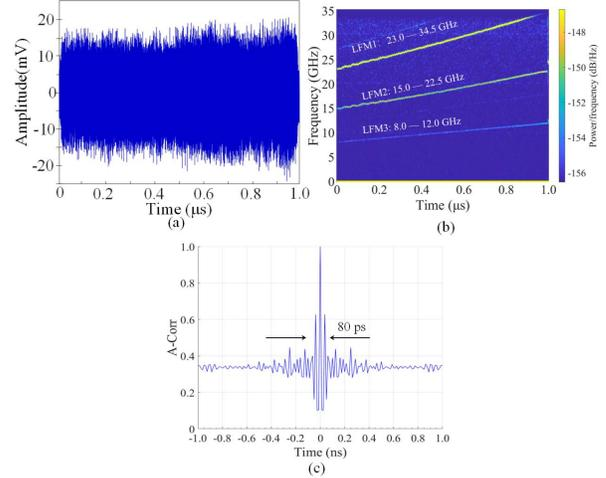
Fig. 5. The generated multi-band LFM signal of Fig. 2(d). (a) the temporal waveform, (b) the instantaneous frequency-time diagram, and (c) the autocorrelation function.
