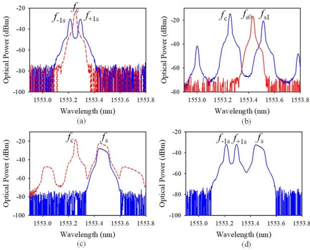
Fig. 2. Optical spectrum at different points of the experiment for multi-band LFM signal illustrated in Fig. 1(a). (a) dotted red line: Point A, solid blue line: Point B; (b) Point D without injection-strength controller; (c) dotted red line: Point D, solid blue line: Point E; and (d) Point F.
