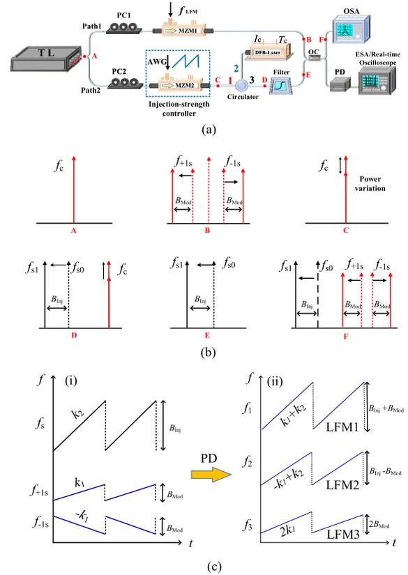
Fig. 1. Basic principle of multi-band LFM signal generation with unidentical bandwidths (a) block diagram, (b) optical spectrum schematic at different stages of block diagram indicated with red points in (a), and (c) the instantaneous frequency-time diagram before (i) and after (ii) PD.
