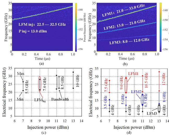
Fig. 6. (a) The generated  $LFM_{inj}$  signal and (b) the multi-band LFM signal with the injected power of 13 dBm; (c) The generated  $LFM_{inj}$  signal and (d) the generated three LFM signals at the output as the injected power is decreased.
