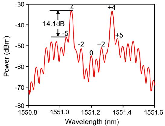
**Fig. 6** The optical spectra at the two outputs of the PBC with a 4-GHz RF signal. The real and dashed lines show the two outputs respectively
