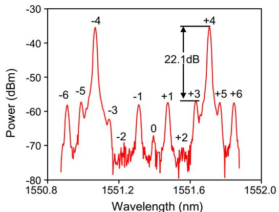
**Fig. 4** The optical spectra at the two outputs of the PBC with a 10-GHz RF signal. The real and dashed lines show the two outputs respectively
