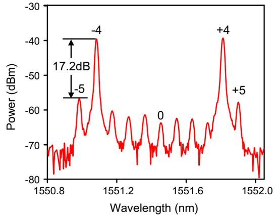
**Fig. 8** The optical spectra at the two outputs of the PBC with an 11.2-GHz RF signal. The real and dashed lines show the two outputs respectively
