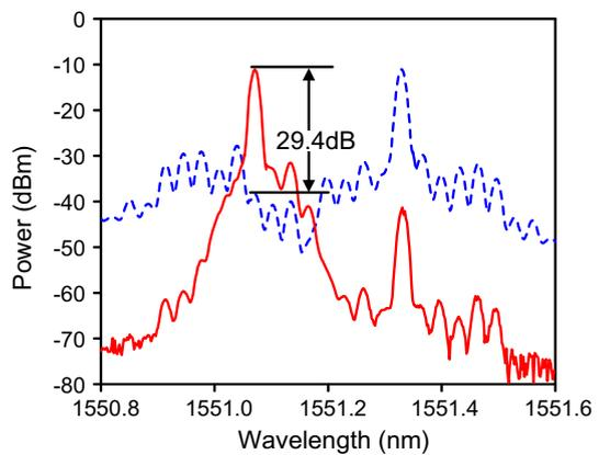
**Fig. 7** The output optical spectrum of the Pol with an 11.2-GHz RF signal
