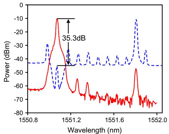
suppressed more than 35.3 dB by the polarization selection. Due to the finite extinction ratio of the modulator, the OSR of the generated signal is limited, but it can be improved by using a modulator with better performance.
