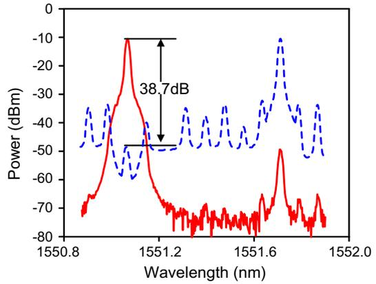
**Fig. 5** The output optical spectrum of the Pol with a 4-GHz RF signal
