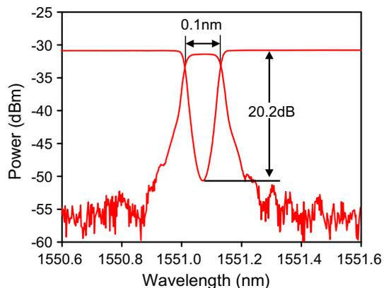
FBG is about 20.2 dB and the 3-dB bandwidth is about 0.1 nm. The FBG can be used to efficiently separate two wavelengths spacing more than 6 GHz.
