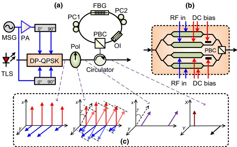
**Fig. 1** a Schematic diagram of the proposed orthogonally polarized dual-wavelength signal generator. b Illustration of the DP-QPSK modulator. c Polarization states of the optical signals
