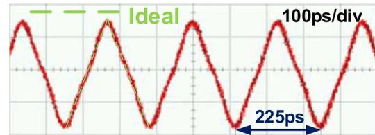
Fig. 4. Measured waveform of the triangular pulse train at the electrical output.
