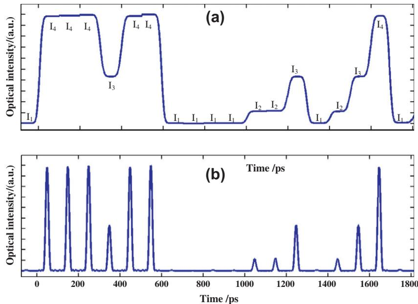
Fig. 4. Temporal waveforms before (a) and after (b) conversion.
