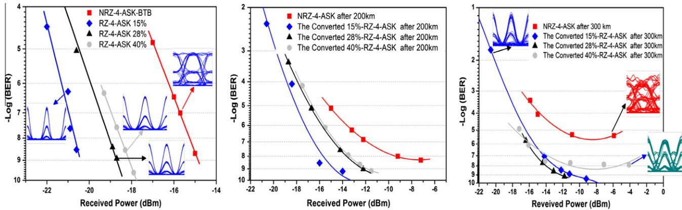
Fig. 5. Measured BER curves (a) BTB NRZ-4-ASK signal and the converted RZ-4-ASK signals, (b) NRZ and the converted RZ signals after 200 km transmission, (c) NRZ and the converted RZ signals after 300 km transmission.
