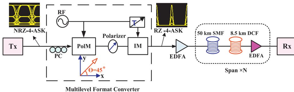
Fig. 1. Set up of the format converter.
