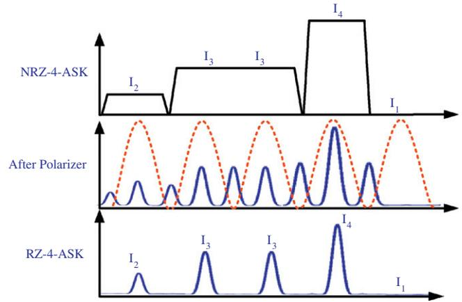
Fig. 2. Operation principle illustration of NRZ 4-ASK to RZ 4-ASK conversion.
