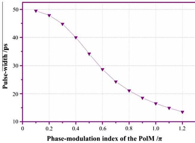
Fig. 3. The influence of the phase-modulation index of PolM on the pulse-width of the converted RZ signal.
