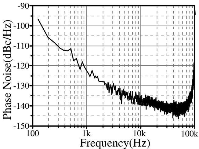
Fig. 3. Phase noise floor of the proposed system at 10 GHz.
