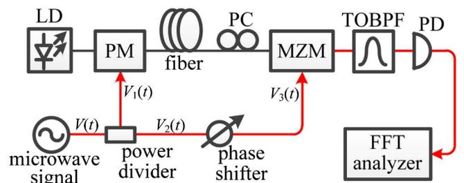
Fig. 1. Schematic diagram of the proposed phase noise measurement system. PC, polarization controller.
