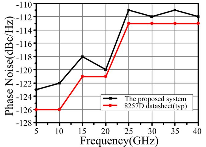
Fig. 5. Phase noises of the wideband signal source (Agilent 8257D) measured by the proposed system and provided by the datasheet (typical value).
