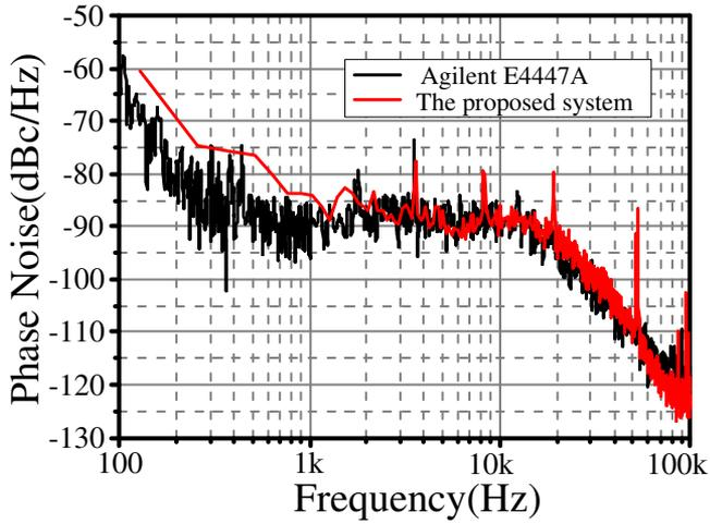
Fig. 2. Phase noise of a 10-GHz clock signal measured by the proposed system (red curve), and that measured by a commercial spectrum analyzer (black curve).
