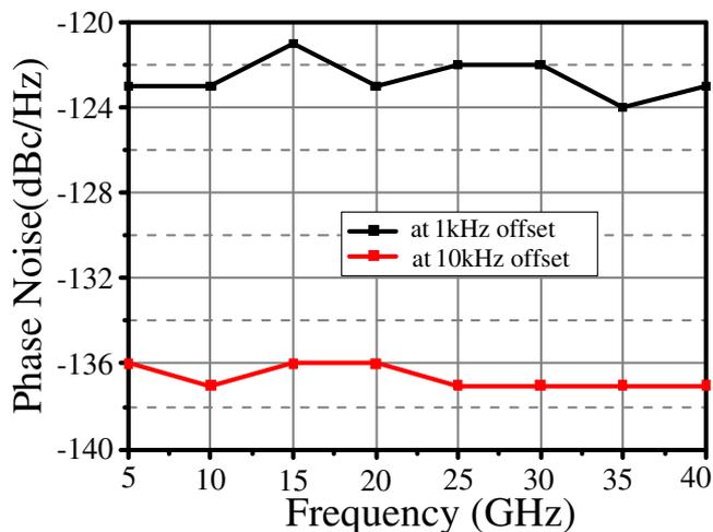
Fig. 6. Phase noise floor at 1- and 10-kHz offset in the frequency range from 5 to 40 GHz.
