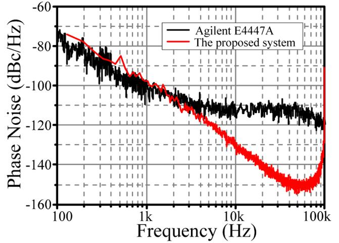
Fig. 4. Phase noise of a 10-GHz OEO measured by the proposed system (red curve), and that measured by the commercial spectrum analyzer Agilent-E4447 (black curve).
