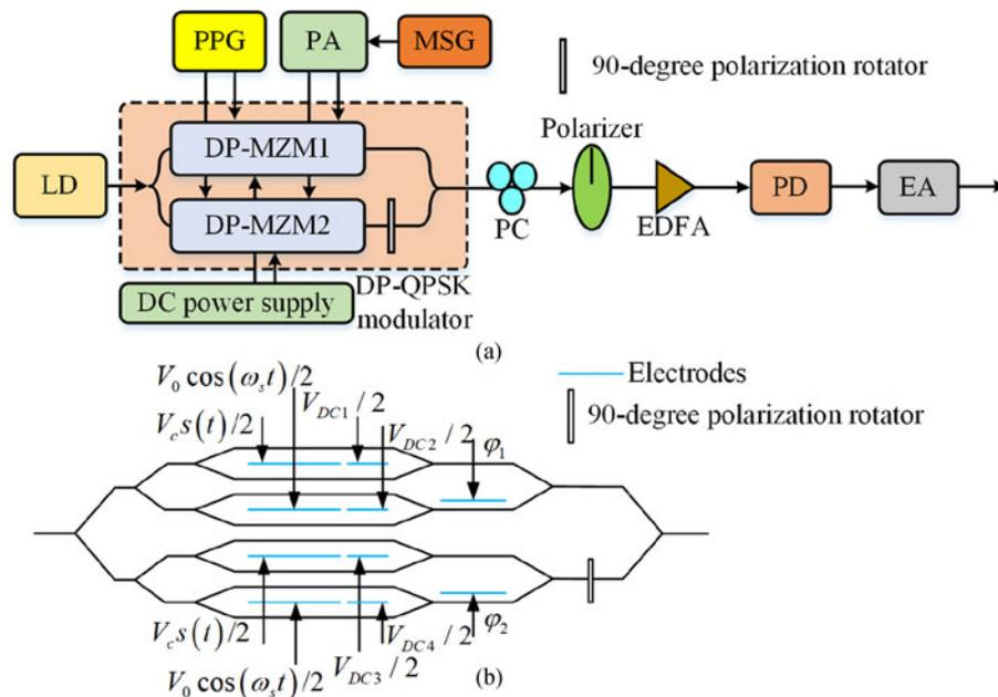
Fig. 1. (a) Schematic diagram of the proposed frequency-tunable phase-coded microwave signal generator. LD, laser diode; DP-MZM, dual-parallel Mach-Zehnder modulator; PC, polarization controller; EDFA, erbium-doped fiber amplifier; PD, photodetector; EA, electrical amplifier; PPG, pulse pattern generator; MSG, microwave signal generator; PA, power amplifier. (b) A diagram of how the electrical signals are applied to the DP-QPSK modulator.
