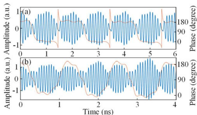
Fig. 12. Temporal waveforms of the generated frequency-quadrupled binary phase-coded microwave signals with carrier frequencies at (a) 10 GHz and (b) 15.8 GHz. The dash lines are the recovered phase information from the waveforms.
