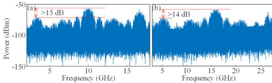
Fig. 8. Electrical spectra of the generated frequency-tripled phase-coded microwave signals with carrier frequencies at (a) 9.99 GHz and (b) 15.9 GHz.
