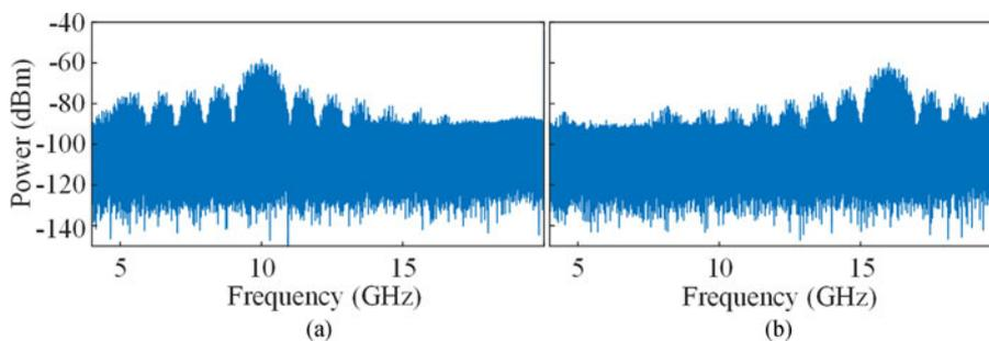
Fig. 5. Electrical spectra of the generated frequency-doubled phase-coded microwave signals with carrier frequencies at (a) 10 GHz and (b) 15.8 GHz.
