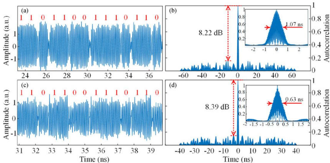
Fig. 4. (a) A section of the generated 64-bit binary phase-coded microwave signal at the fundamental frequency of 10 GHz. (b) Autocorrelation of the generated phase-coded microwave signal in (a). (c) A section of the generated 64-bit binary phase-coded microwave signal at the fundamental frequency of 15.8 GHz. (d) Autocorrelation of the generated phase-coded microwave signal in (c). The insets in (b) and (d) are the zoom-in views of the autocorrelation peaks.
