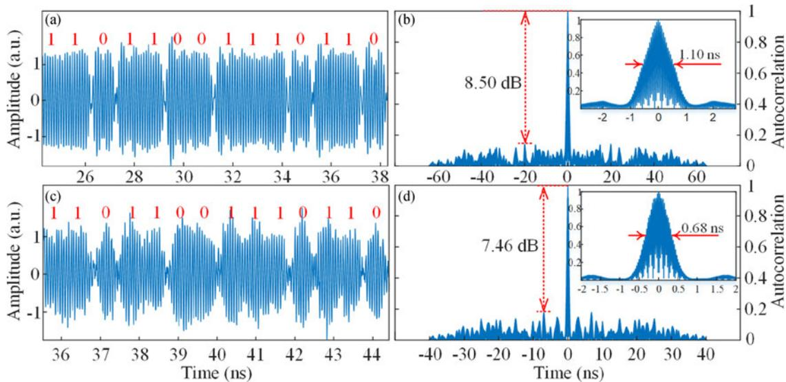
Fig. 10. (a) A section of the generated 64-bit frequency-tripled binary phase-coded microwave signal at 9.99 GHz. (b) Autocorrelation of the generated phase-coded microwave signal in (a). (c) A section of the generated 64-bit frequency-tripled binary phase-coded microwave signal at 15.9 GHz. (d) Autocorrelation of the generated phase-coded microwave signal in (c). The insets in (b) and (d) are the zoom-in views of the autocorrelation peaks.
