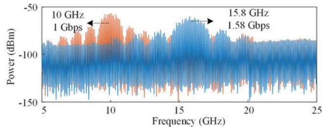
Fig. 2. Electrical spectra of the generated 10 GHz and 15.8 GHz binary phase-coded microwave signals at the fundamental frequency.
