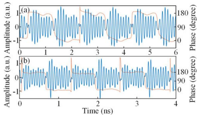
Fig. 6. Temporal waveforms of the generated frequency-doubled binary phase-coded microwave signals with carrier frequencies at (a) 10 GHz and (b) 15.8 GHz. The dash lines are the recovered phase information from the waveforms.
