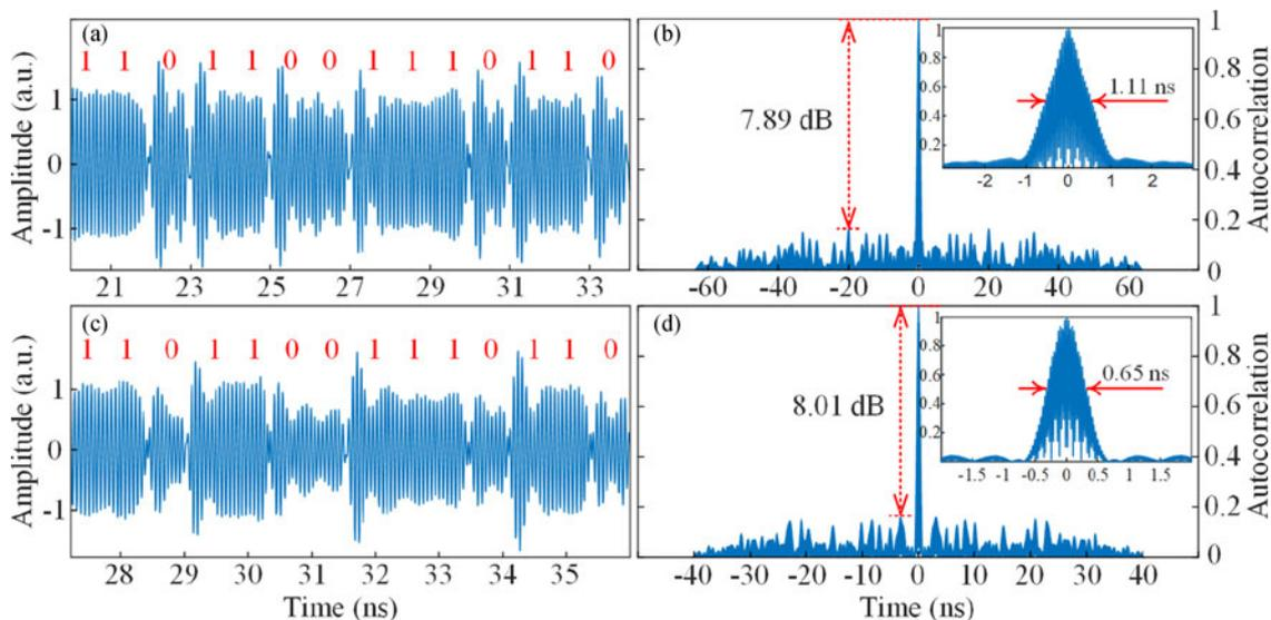
Fig. 7. (a) A section of the generated 64-bit frequency-doubled binary phase-coded microwave signal at 10 GHz. (b) Autocorrelation of the generated phase-coded microwave signal in (a). (c) A section of the generated 64-bit frequency-doubled binary phase-coded microwave signal at 15.8 GHz. (d) Autocorrelation of the generated phase-coded microwave signal in (c). The insets in (b) and (d) are the zoom-in views of the autocorrelation peaks.
