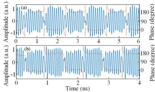
Fig. 3. Temporal waveforms of the generated fundamental binary phase-coded microwave signals with carrier frequencies at (a) 10 GHz and (b) 15.8 GHz. The dash lines are the recovered phase information from the waveforms.
