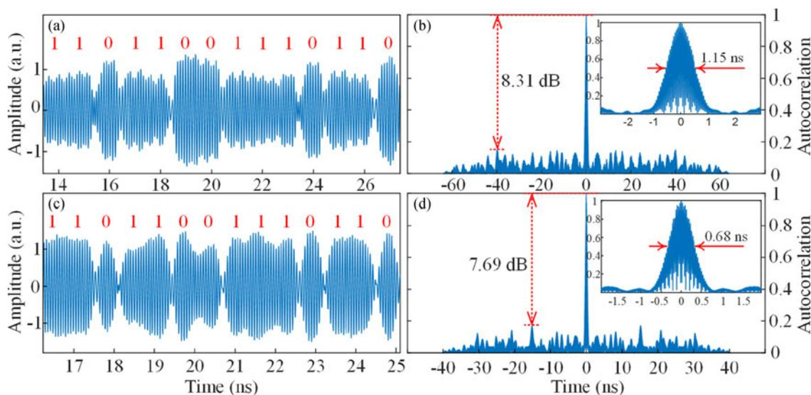
Fig. 13. (a) A section of the generated 64-bit frequency-quadrupled binary phase-coded microwave signal at 10 GHz. (b) Autocorrelation of the generated phase-coded microwave signal in (a). (c) A section of the generated 64-bit frequency-quadrupled binary phase-coded microwave signal at 15.8 GHz. (d) Autocorrelation of the generated phase-coded microwave signal in (c). The insets in (b) and (d) are the zoom-in views of the autocorrelation peaks.
