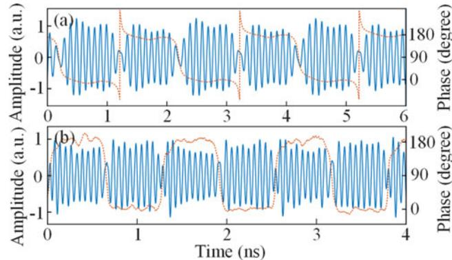
Fig. 9. Temporal waveforms of the generated frequency-tripled binary phase-coded microwave signals with carrier frequencies at (a) 9.99 GHz and (b) 15.9 GHz. The dash lines are the recovered phase information from the waveforms.
