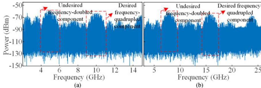
Fig. 11. Electrical spectra of the generated frequency-quadrupled phase-coded microwave signals with carrier frequencies at (a) 10 GHz and (b) 15.8 GHz.
