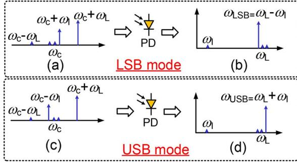
Fig. 2. Illustrations of the (a), (c) optical spectra of the optical CS-SSB-modulated signals at the output of the DPMZM in the LSB and USB modes; and (b), (d) the corresponding electrical spectra.
