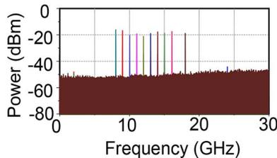
Fig. 6. Electrical spectra of the single-sideband mixer in the LSB mode when the IF frequency is fixed at 2 GHz and the LO frequency tuned from 10 to 20 GHz.
