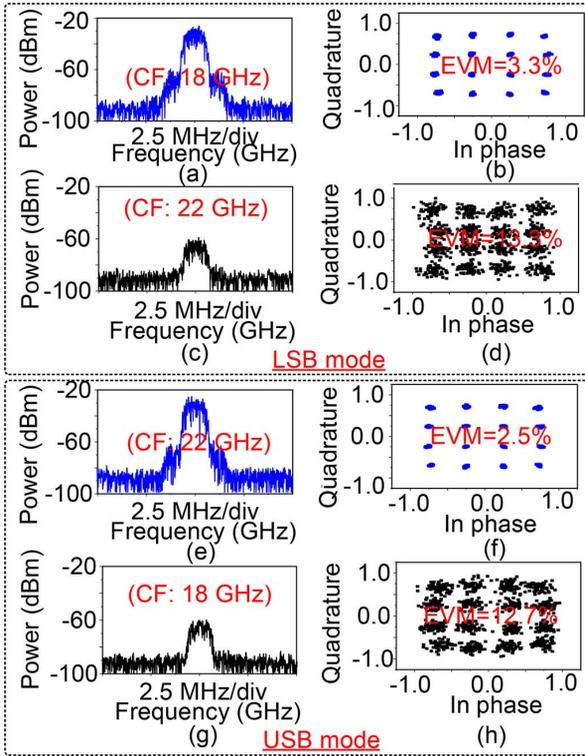
Fig. 4. Electrical spectra and constellations of the (a), (b) LSB signal and (c), (d) USB signal when working in the LSB mode, and (e), (f) USB signal and (g), (h) LSB signal when working in the USB mode.
