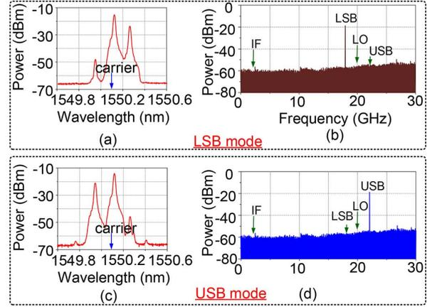
Fig. 3. (a), (c) Optical spectra of the signals at the output of the DPMZM when the single-sideband mixer is working in the LSB and USB modes; and (b), (d) the corresponding electrical spectra (RBW = 8 MHz).
