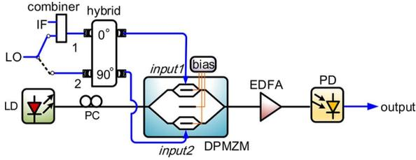
Fig. 1. Schematic diagram of the photonic microwave single-sideband mixer.
