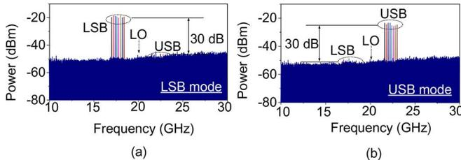
Fig. 5. Electrical spectra of the single-sideband mixer in the (a) LSB and (b) USB modes when the IF frequency increases from 1.6 to 3 GHz.
