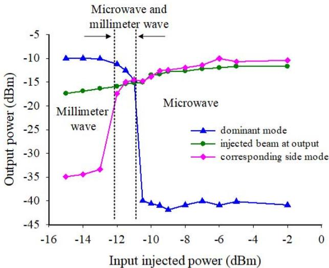
Fig. 3. Effect of input injected beam power on power of output dominant mode, injection mode and corresponding mode for generation of different band of frequencies for wavelength detuning of  $-0.13$  nm.
