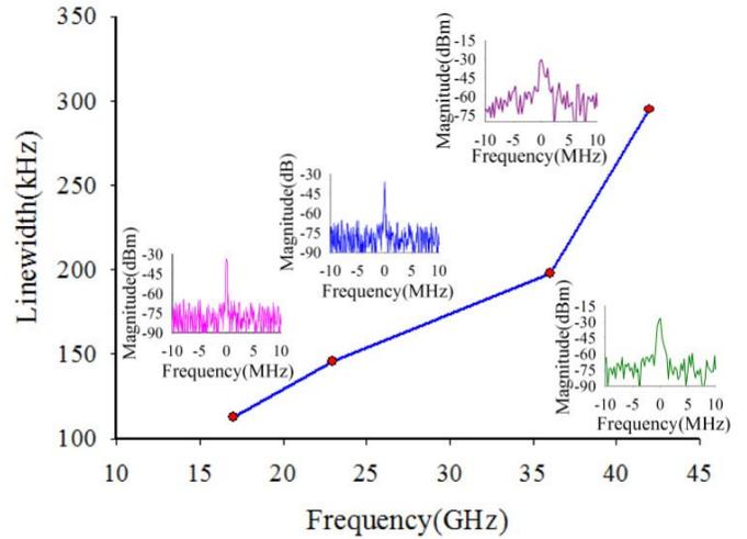
Fig. 7. Linewidth and power spectra of generated multiband (Ku-, K-, Ka-, and V-band) RF signal.
