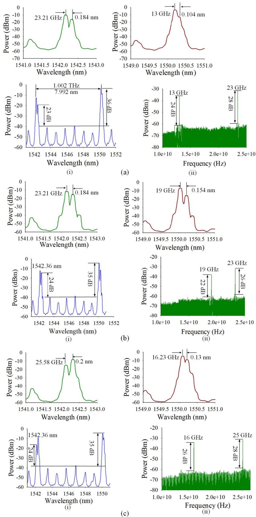
Fig. 4. Optical and electrical spectra with different wavelength detuning corresponding to the dominant mode and the seventh mode for generating two frequencies. (a) 0.184 and 0.104 nm corresponding to the frequency of 23 and 13 GHz. (b) 0.184 and 0.154 nm corresponding to the frequency of 23 and 19 GHz. (c) 0.2 and 0.13 nm corresponding to the frequency of 25 and 16 GHz.
