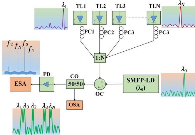
Fig. 1. Experimental setup of the proposed multiband frequency generator. ESA: electric spectrum analyzer; OSA: optical spectrum analyzer; PD: photo detector; OC: optical circulator; CO: coupler; PC: polarization controller; TL: tunable laser.
