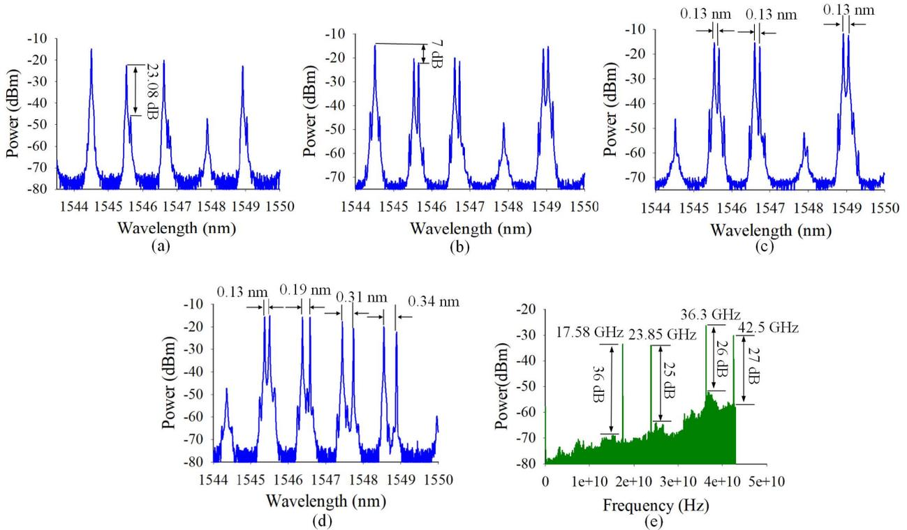
Fig. 5. Output results. (a) Millimeter wave with three injected beam with constant wavelength detuning. (b) Millimeter and micrometer. (c) Microwave with the same wavelength detuning of  $-0.13$  nm. (d) Microwave generation with four injected beams with different wavelength detuning. (e) Electrical output of generated signal, which corresponds to the optical output of (d).
