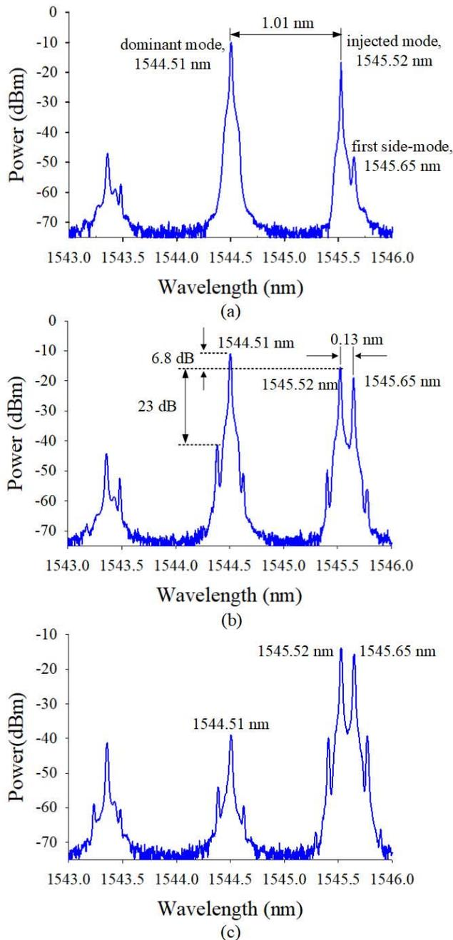
Fig. 2. Optical spectrum with single beam injection with negative wavelength detuning of  $-0.13$  nm using different injected power that generates. (a) Millimeter wave. (b) Microwave and millimeter wave. (c) Microwave.
